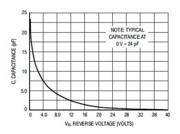
Figure 2. Typical Capacitance
